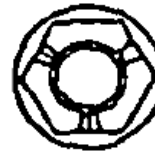
Prevailing torque surface
