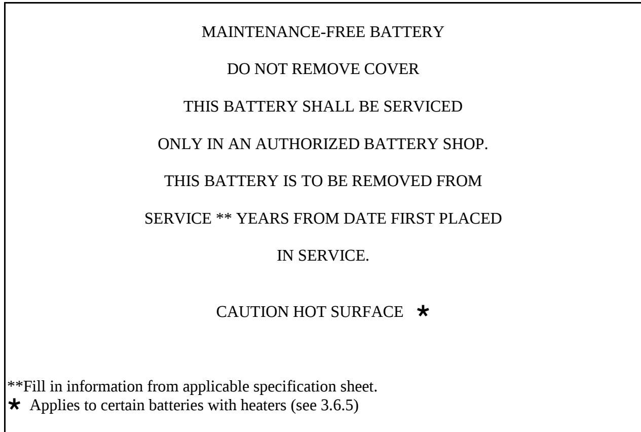
FIGURE 2. Battery caution marking.
