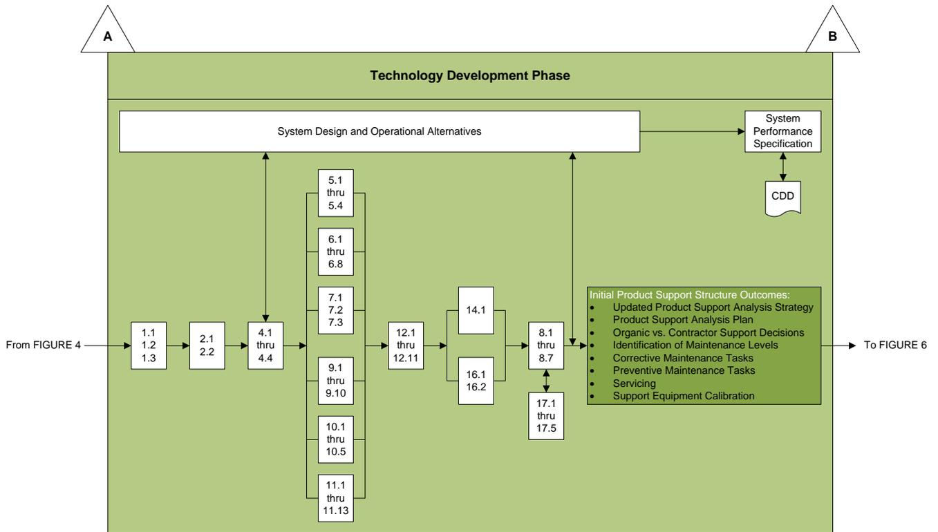
FIGURE 5. Conventional PSA process flow for TD phase
