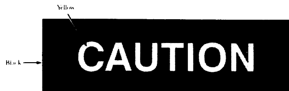
Figure 6-16. Example of a Caution Sign (Ref. 21)
