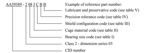
AA59589 - 2 08 J C B B indicates: boundary dimension series 03; bore diameter 40 mm, outside diameter 90 mm, width 23 mm; pressed steel cage; single shield on filling slot side; ABEC-1 tolerance class, normal radial internal clearance; filled with grease in accordance with MIL-PRF-81322.
